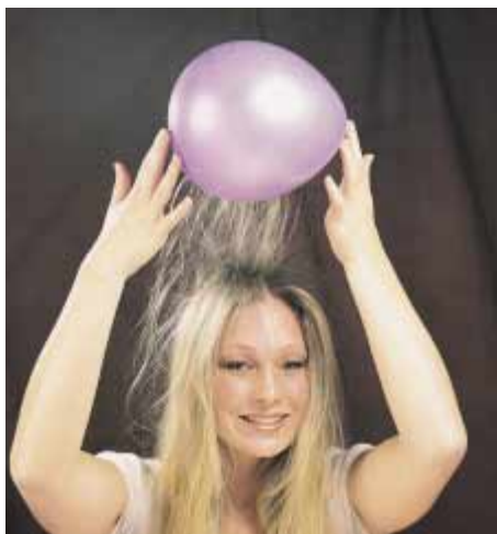
Figure 23.2 Rubbing a balloon against your hair on a dry day causes the balloon and your hair to become charged.
